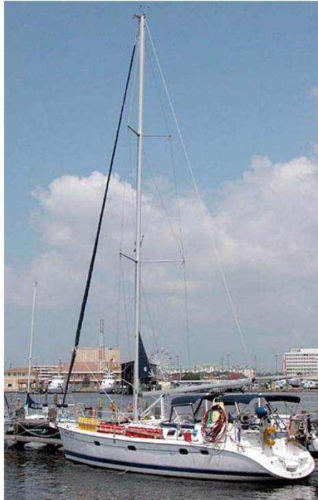
Figure 5. The *Summer Breeze*, a 46' sloop, which served as the research vessel for the 2005 MPS cruise (Photo: Bill Lang). To extend the reach of the vessel, 34 red and yellow jerry cans were lashed to the deck. One of the towed hydrophones can be seen coiled up at the port stern.
